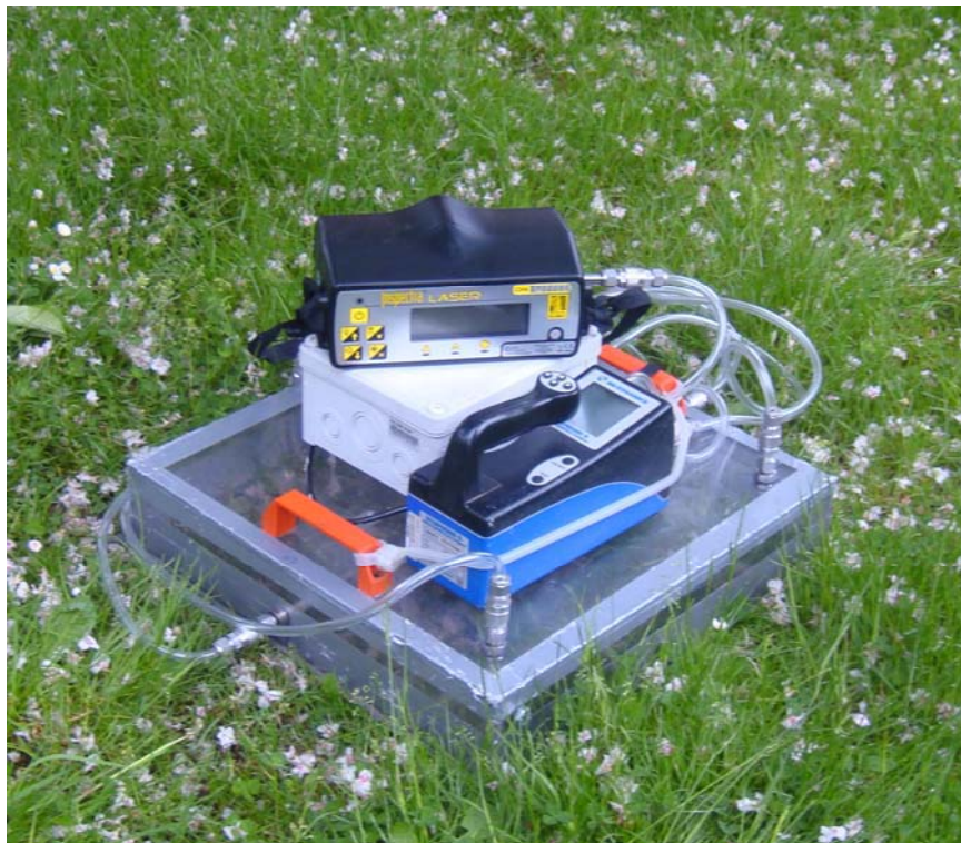
Figure 2. Closed dynamic chamber system connected to Ecoprobe5® and Inspectra® Laser.
